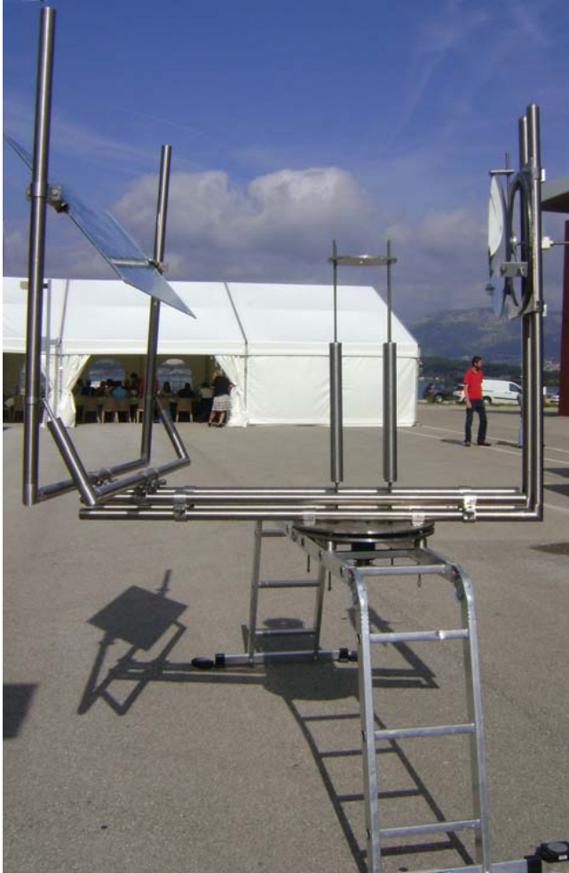
Solar oven of 5kW (16m2 of mirror) planned on the domain of this chalet, visible from June 2010.
